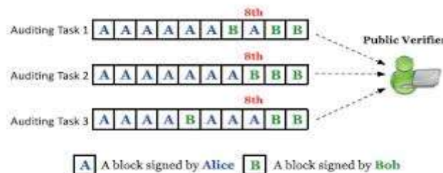
Fig. 1: A and B share a data file in the cloud, and public verifier audits shared data integrity with existing mechanisms
